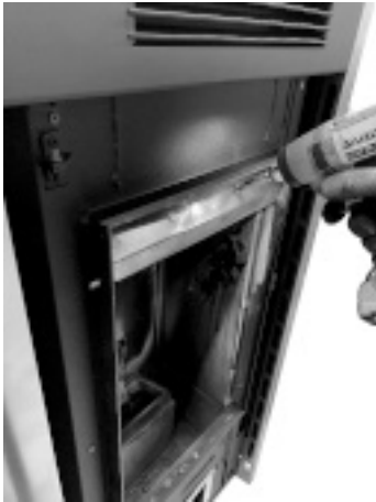
Fig. 46 - Remove the deflector
