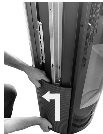
Fig. 25 - Remove the lower plate
