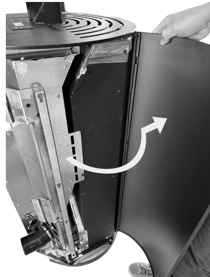
Fig. 20 - Release upper panel
